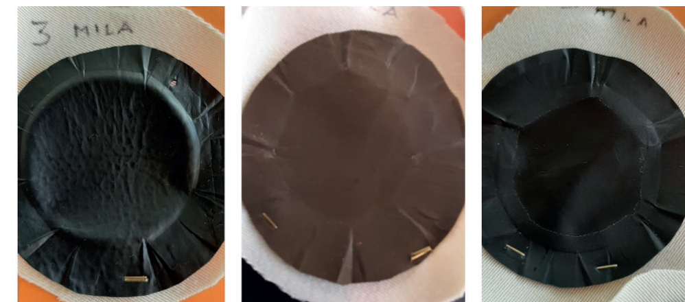
Figure 14 Mycelium-materials tests for ensuring their suitability for application in car interiors
