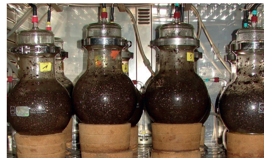
Figure 24 Biodegradability and compostability tests performed by Normec OWS
