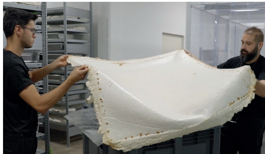
Figure 19 Harvested 1 sqm SLF panels, ready for drying at MOGU's facility
