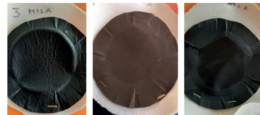
Figure 17 Mycelium-materials tests for ensuring their suitability for application in car interiors, performed by CRF and Volkswagen Group
